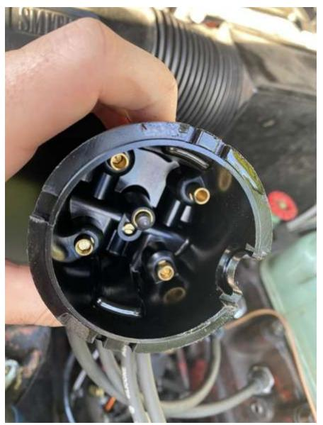
No signs of carbon tracking or arcing meant the cap was okay. Another sign suggesting the points.
