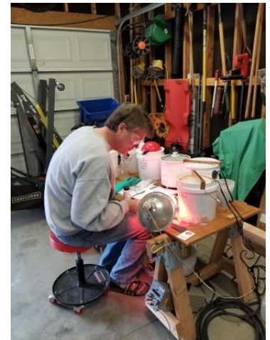
At the plating station: Acid, baking soda, RO water, degreaser, RO water, plating.... Repeat.
