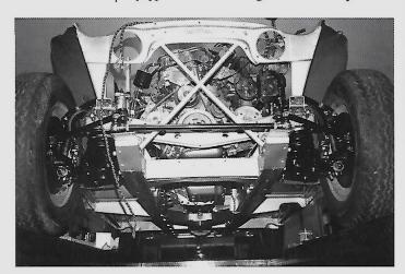
The most frustrating part of an engine swap is working out the gear ratios. later 240Zs with five-speed transmissions have ratios nearly identical to the 3000's four-speed-box with overdrive. Transmission fits nicely into the Healey mount positions align with the Healey chassis, requiring only a slight bracket alteration to use the original rubber mount pads.
