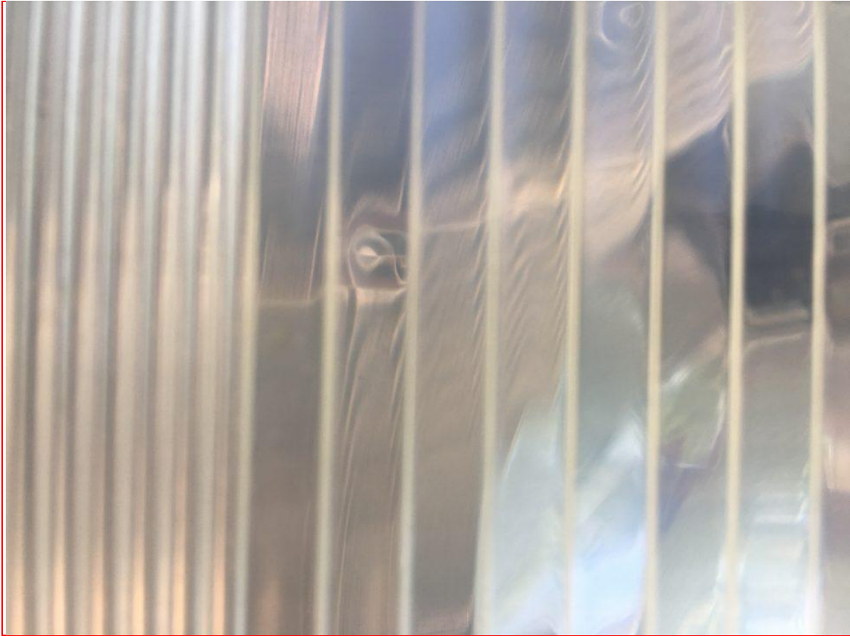
Making progress – here is a close-up of the lens surface after the 1500 grit.
