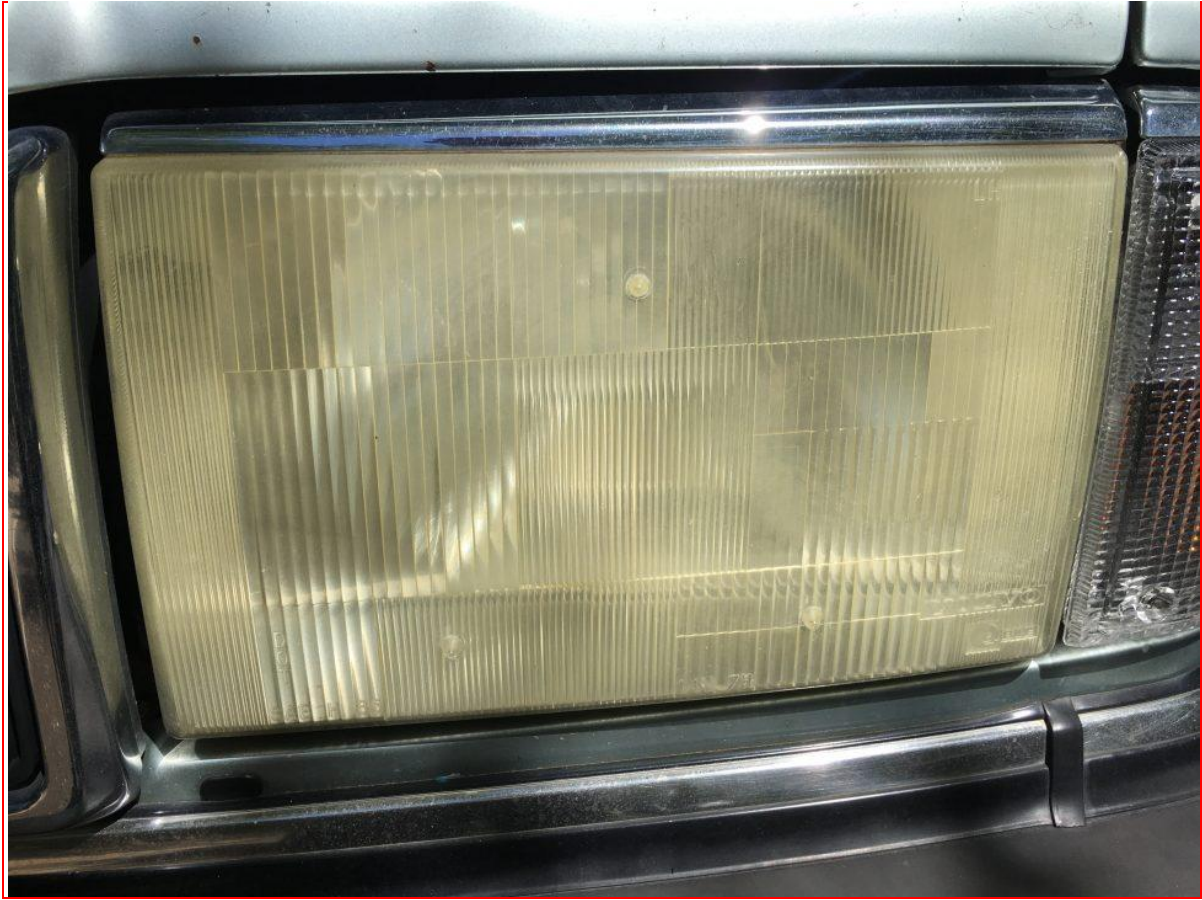
Starting Point – oxidized and yellowed lens
