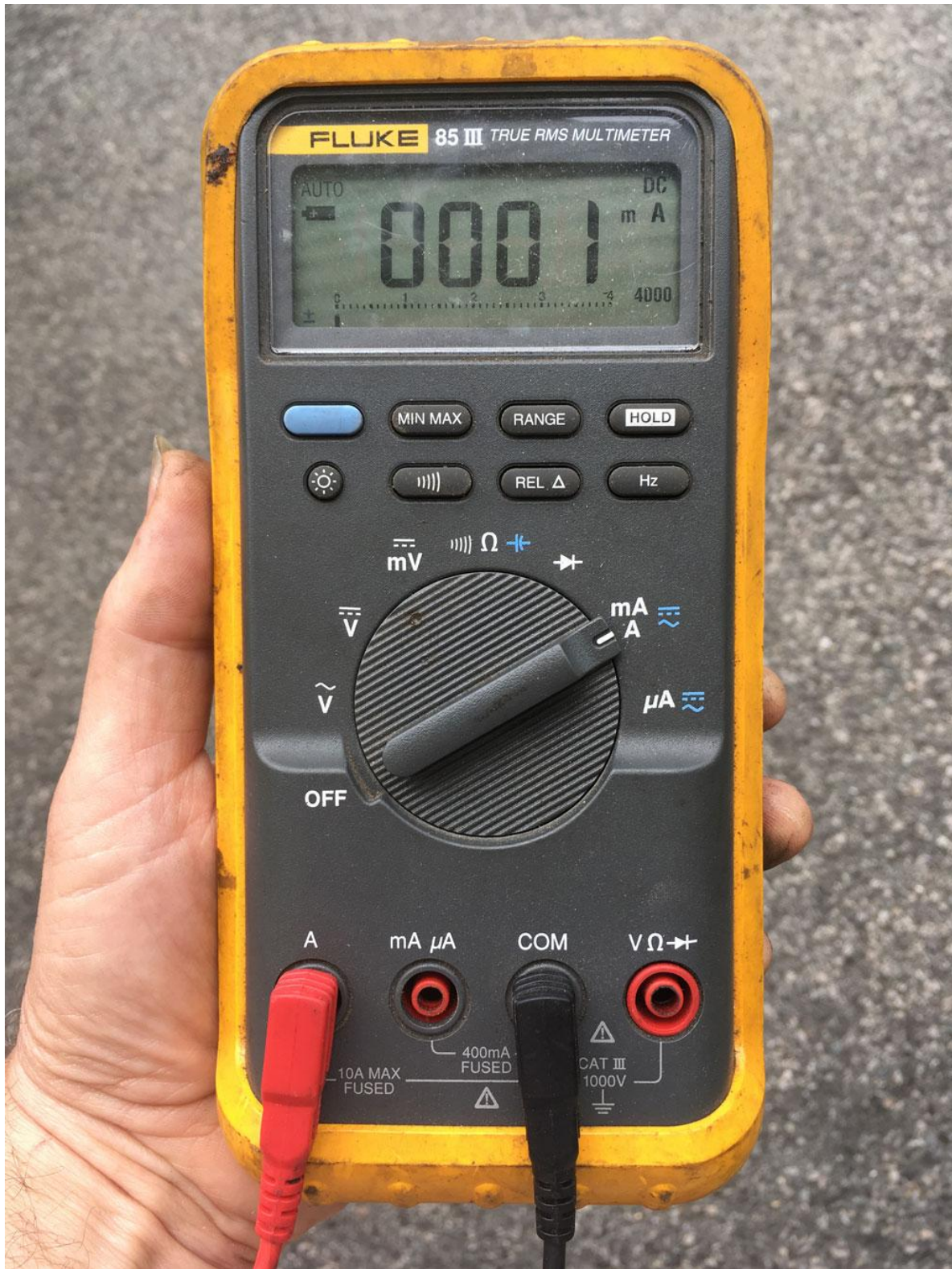
A multimeter configured to measure current on the high amperage setting (red probe in the “A” socket, rotary dial turned to the A setting)
