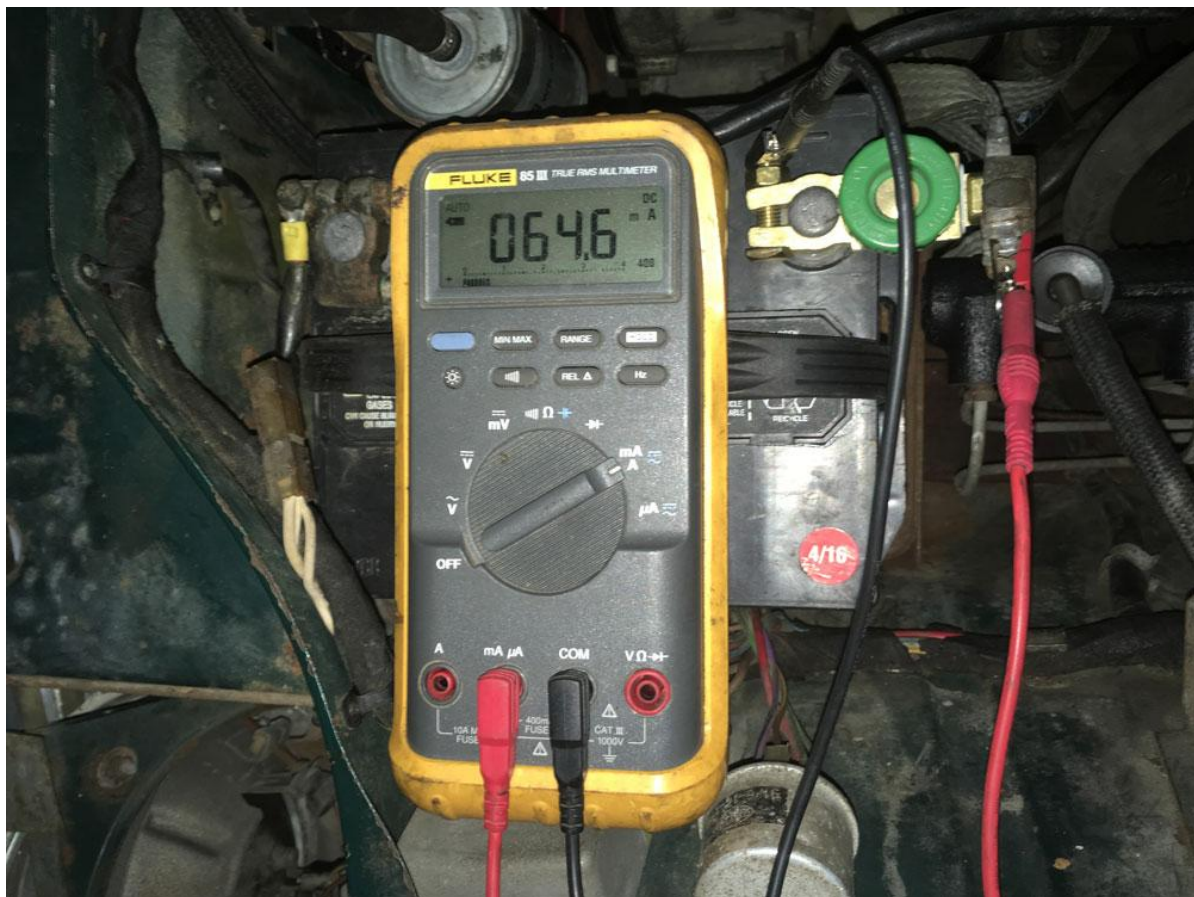
A battery with a battery disconnect switch (green knob) installed, and the meter connected across the disconnect switch, between the battery negative terminal and ground
