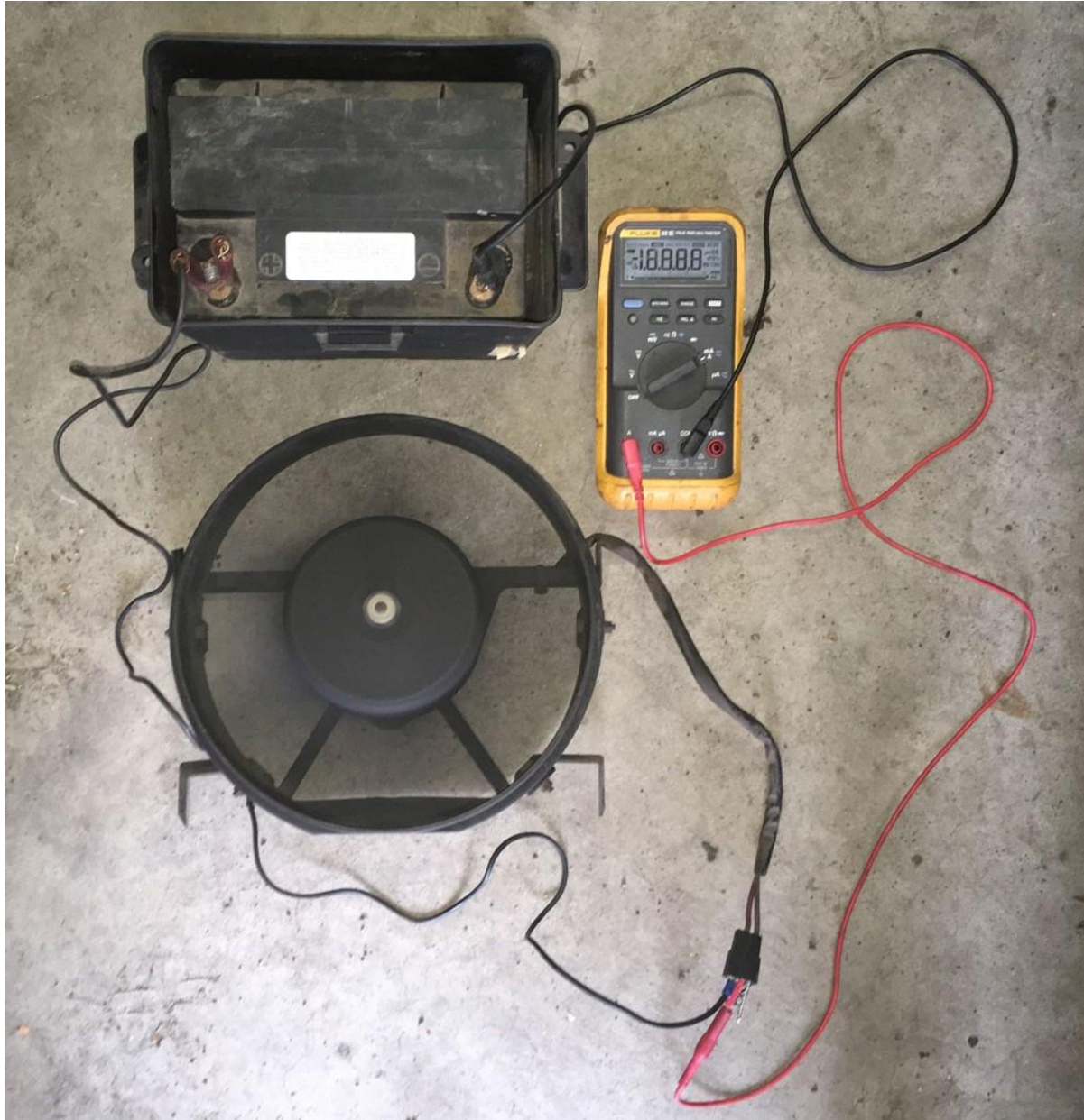
Meter in series in a real circuit, measuring current
