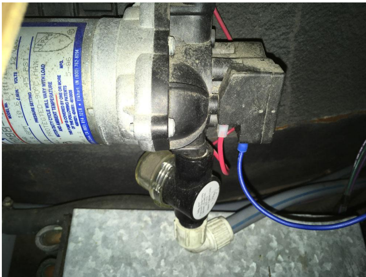
Hot-wiring an electric motor directly to the battery
